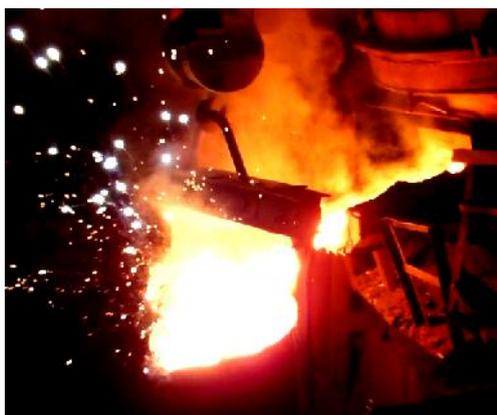
The process of cast iron desulphurization by means of magnesium that is reduced from the oxide in the volume of melt due to the heat of parallel chemical transformations in ladle furnace
